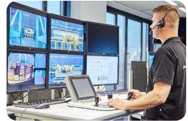
Remotely operated STS cranes
