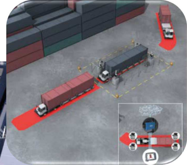
Environmental perception on terminal tractors
